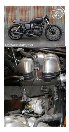
Step 6: The carburetors and intake manifolds should be easy to access at this point. Remove all the hoses from the carburetor and manifold and follow them back to the charcoal box. (charcoal canister)
