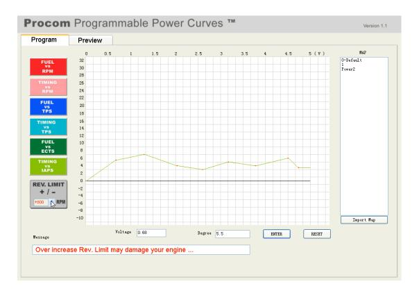
After editing the colored functional data, if you intend to change your machine's Revolution Limit, then you can go to the grey "REV. LIMIT" section and click the up/down arrows to increase/decrease the revolution limit as you desire. The maximum increment/decrement is +3000/-3000RPM. The value you selected to appear in the box will be automatically saved if you go to the next step.
