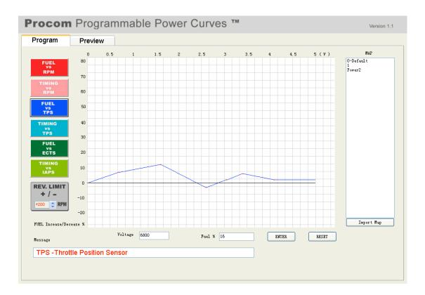
After you have finished creating one function data, such as, FUEL vs. RPM, then you just click the left colored function button to start creating a new function data, such as, FUEL vs. TPS. The previous function data you have just created is automatically saved.
